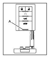
To remove the key, press the button (A) near the bottom of the keyless access transmitter, and pull the key out. Never pull the key out without pressing the button.
